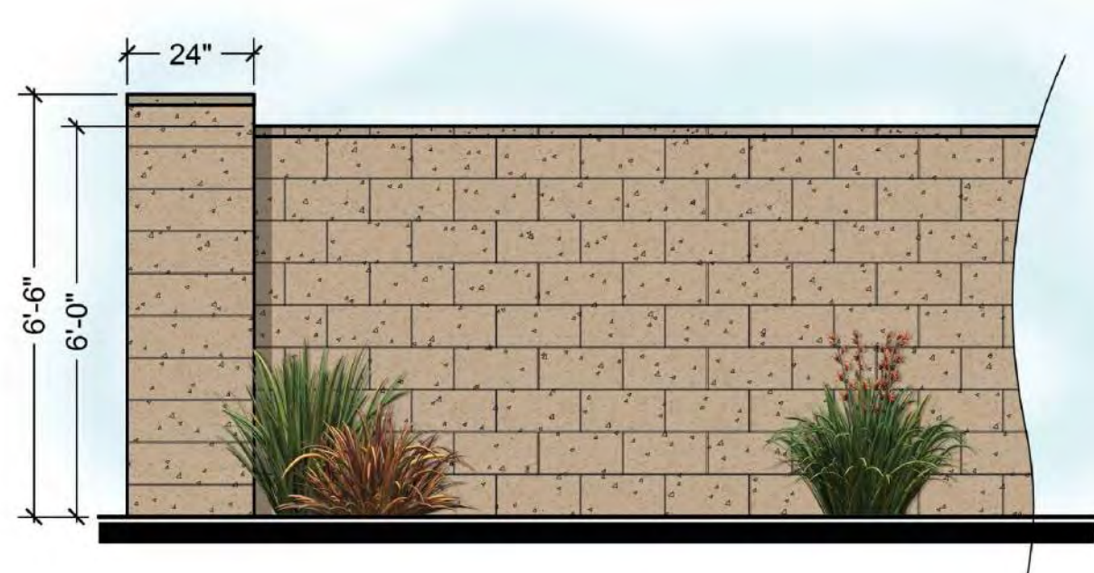
W-01 & W-02 6'-0" TALL SPLIT-FACE DECORATIVE BLOCK WALL W/ 2" THICK SPLIT-FACE CAP SCALE : 3/8" = 1'-0"
